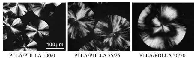
Figure 4. POM micrographs of PLLA/PDLLA blends melt-crystallized at 140 °C.
